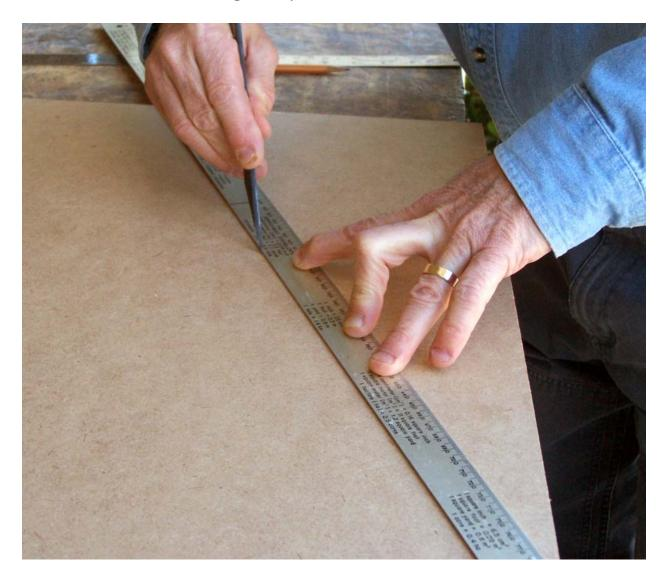
You now have your triangle marked out. It should be exactly what we drew earlier. The working edge (side 1) should be 22 inches in length and the opposite side (side 2) should be a bit less than 9 1/8 inches in length. This will give us an angle of 22 1/2 degrees.
