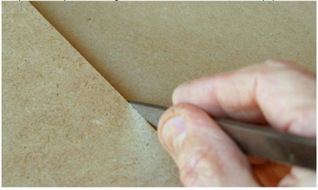
Now, move the template upwards so that the edge that was against the ruler is now aligned with that knife mark, while keeping the point on the
