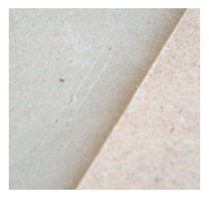
If the error is too large (maybe 5/16 inch), you'll have to re-cut the template to make the angle smaller. Remember that the error shown is 8 times the actual error so don't cut too much off at a time. And when you make the cut, make sure that you cut all the way along the edge or you won't have a straight edge - you'll have a bent edge.
