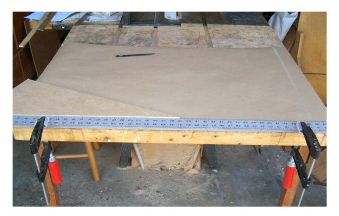
Align the point of your template with one of the marks on the ruler, and the make sure the edge is tight against the ruler. Here, I'm using the 29 inch mark for the point but that's totally arbitrary.
