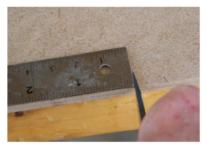
Now, mark a line upward from this 22 inch mark using the combination square.
