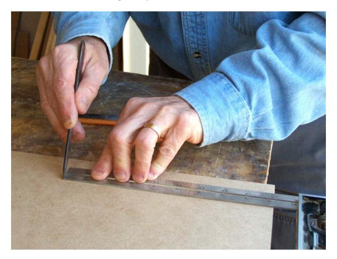
Now, using a straightedge, mark a line from the corner of the hardboard to the mark you just made.
