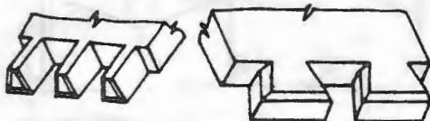
Do not apply excessive quantities of glue to the mating parts of the joint. If it is a good fit, much of the glue will be pressed out as it comes together, making it necessary to wipe surplus glue away with a damp rag. If the interior faces are to be polished or varnished, it is worthwhile to give them at least a first coat before assembly. Surplus glue can then be more readily removed and staining of the wood will be avoided.
