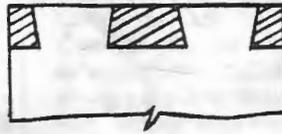
Joiner's joint with neater and smaller pins - perhaps for his tool chest or a kitchen fitment. Slope 1 : 6 or 1 : 8 according to timber used.
