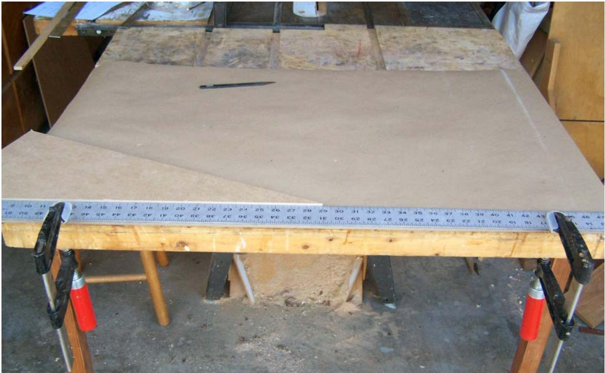
Align the point of your template with one of the marks on the ruler, and the make sure the edge is tight against the ruler. Here, I'm using the 29 inch mark for the point but that's totally arbitrary.
