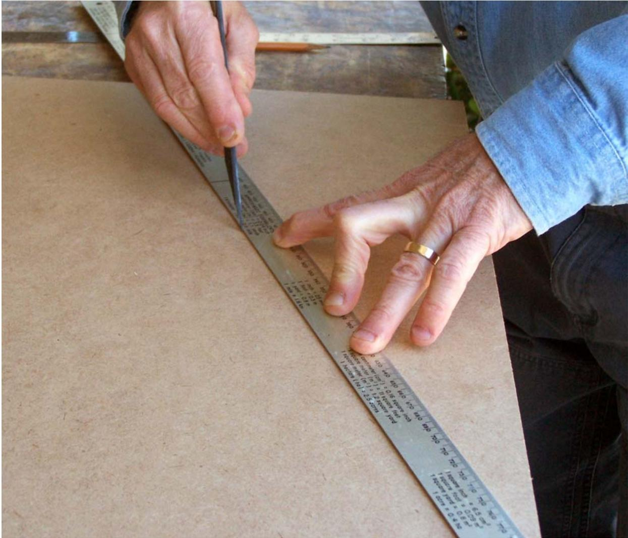
You now have your triangle marked out. It should be exactly what we drew earlier. The working edge (side 1) should be 22 inches in length and the opposite side (side 2) should be a bit less than  $9 \frac{1}{8}$  inches in length. This will give us an angle of  $22 \frac{1}{2}$  degrees.
