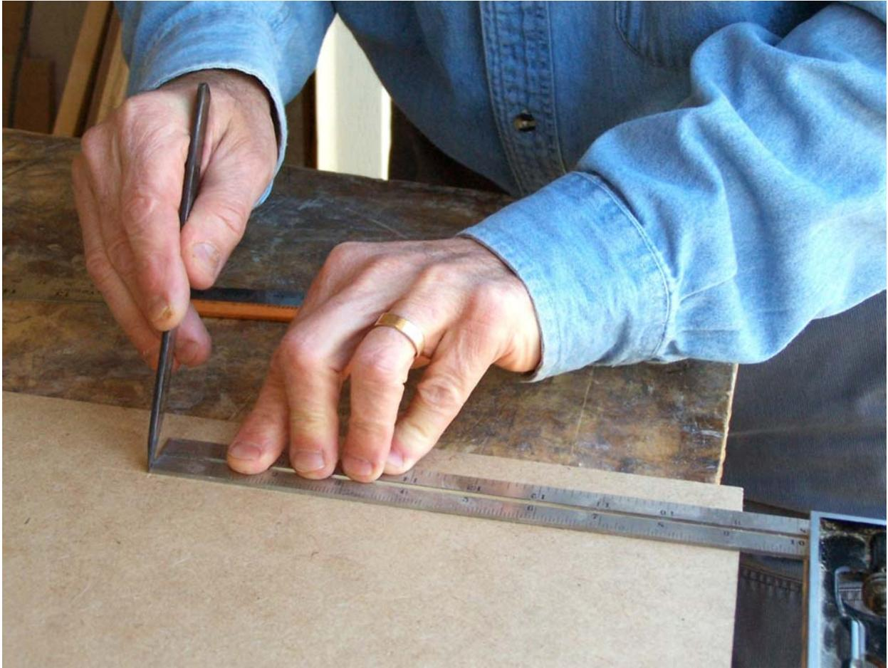
Now, using a straightedge, mark a line from the corner of the hardboard to the mark you just made.
