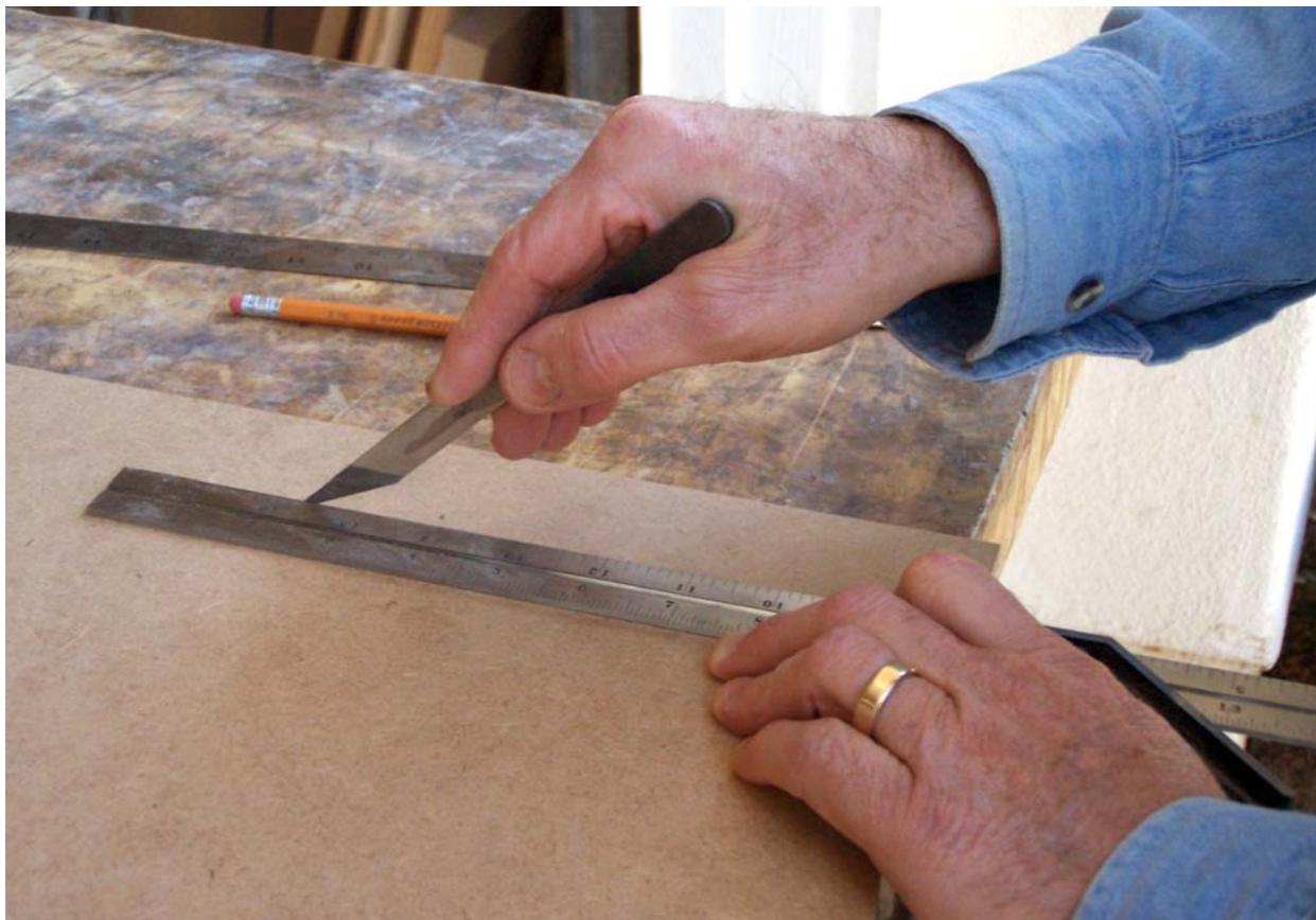
Then put a mark a bit less than 9 1/8 inches from the working edge.
