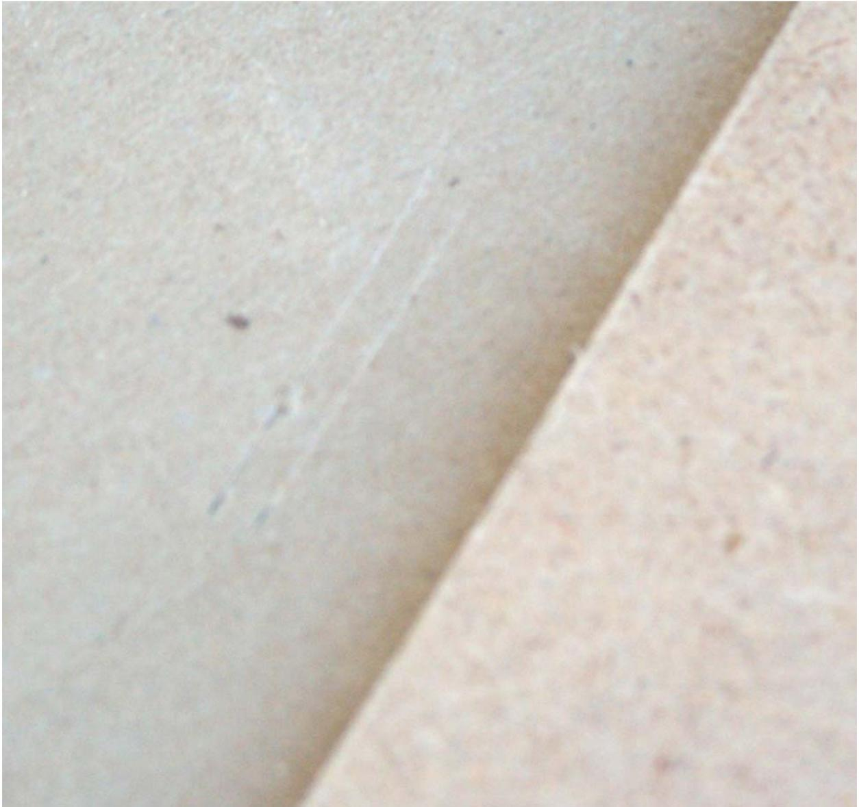
If the error is too large (maybe  $\frac{5}{16}$  inch), you'll have to re-cut the template to make the angle smaller. Remember that the error shown is 8 times the actual error so don't cut too much off at a time. And when you make the cut, make sure that you cut all the way along the edge or you won't have a straight edge - you'll have a bent edge.
