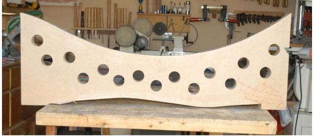
Note the recurve on one end, which is just a decorative effect. The recurve should never hit the floor because it will stop the rocker too abruptly.
