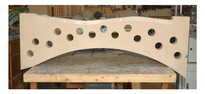
When using a form like this, use clamps and clamp the form to your bench. It will get quite heavy with all the clamps and will fall over unless clamped to the bench.
