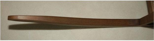
I also did a buildup where the legs will attach to the rockers. I did this by gluing some additional laminates at those locations.
